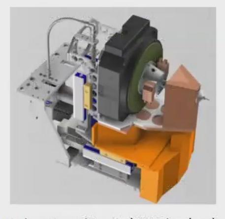
Air-bearing phi-axis (360 deg/sec) Air-bearing sample z stage (up to 300 mm/s) Low profile SMARACT stages
