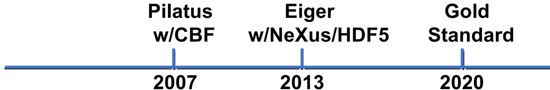
DECTRIS Ltd has dominated the market for MX detectors, first with Pilatus detectors using CBF since 2007 and recently with Eiger detectors using NeXus/HDF5 since 2013. The Gold Standard is a common set of metadata for both imgCIF/CBF and NeXus/HDF5 NXmx which helps the community to follow Findability, Accessibility, Interoperability and Reusability (FAIR) principles.
